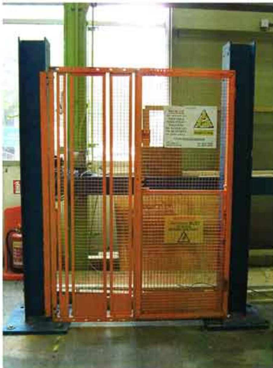
Figure A1: Fullgate lift shaft safety gate system installed in BRE test rig
