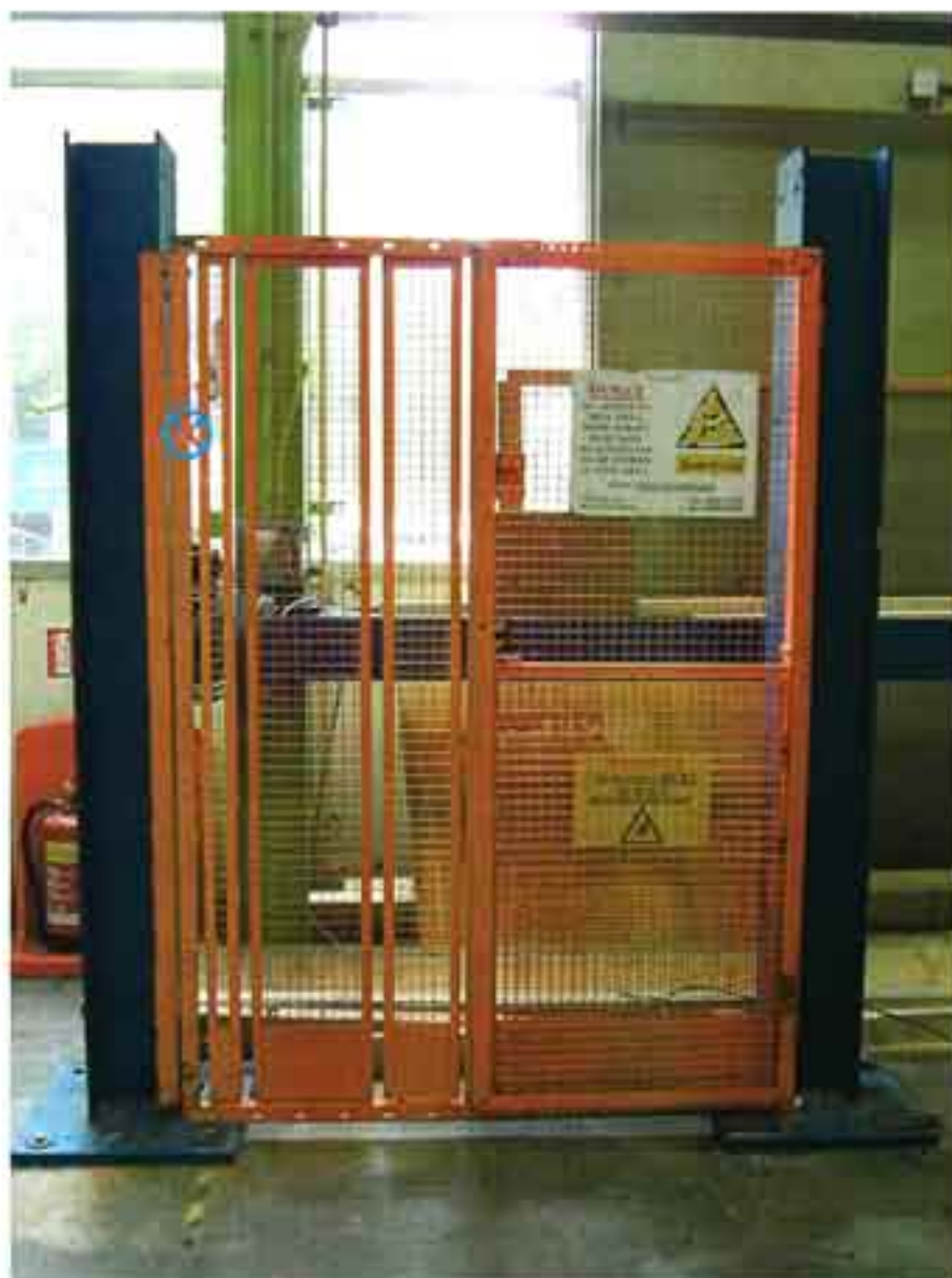
Figure A6: Safety gate pull-out test loading location
