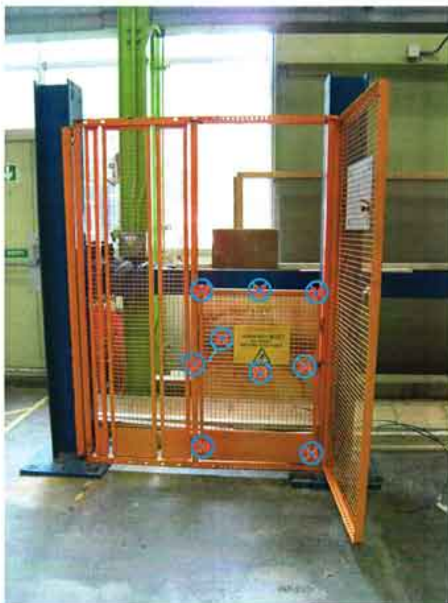
Figure A4: Horizontal static load test locations with main door open
